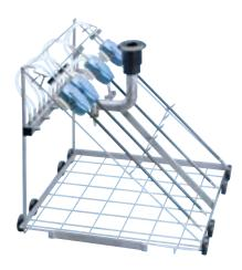
The E 428 load carrier is designed for use in the PG 8536 washer-disinfector. It accommodates 6 EndoWrist instruments with a shaft diameter of 8 mm. Two connections are available for each of these instruments, allowing the separate irrigation of the control housing and the shaft interior, including the critical distal end.
